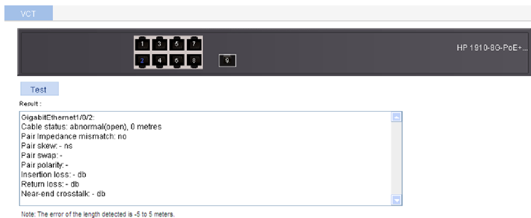
Figure 80 Testing the status of the cable connected to an Ethernet port
